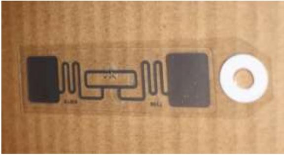
*This image is an Alien H3 9662 Inlay, laminated with a reinforcement ring that forms the reusable tag. 500 Tags will be enough to double tag all runners until we need to expand beyond 250 runners in a race.*
