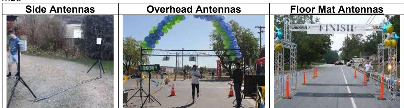
After much research we have found that the best solution for our events is to use a 4-metre floor mat antenna setup, this requires a 4-port fast RFID Reader to capture the runner's tags as they cross the finish line.
